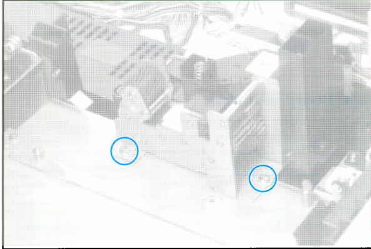
Figure 6-18 Main Motor Removal
